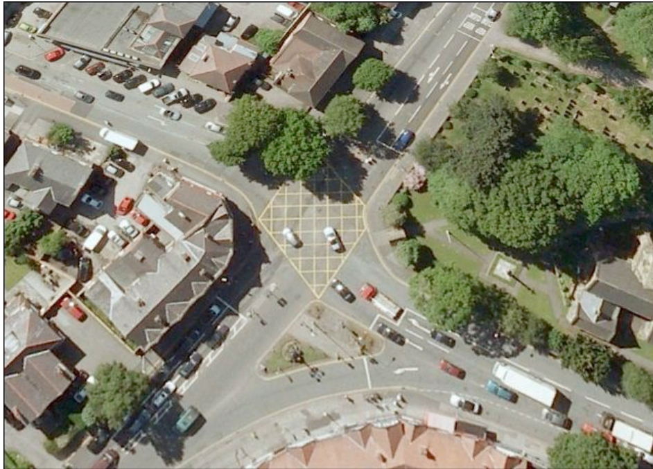
Fig. 1 Poynton, Stockport; The traffic signal controlled layout and local environment prior to the works of 2012. This junction handles 27,000 vehicle movements per day
